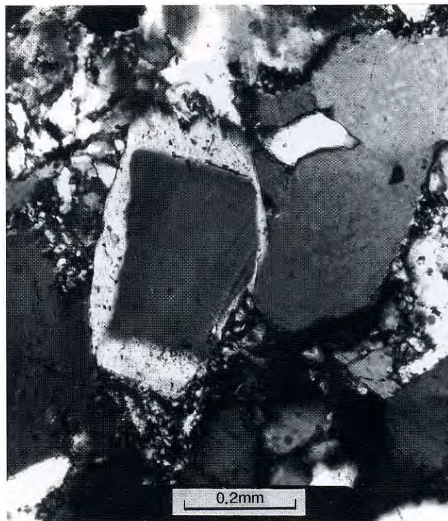
Fig. 9. Overgrowth of K-feldspar on feldspar grain in the sandstone of the Bjorøy Formation.
